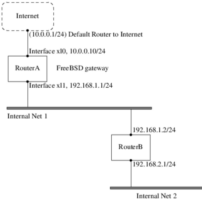
In this scenario, **RouterA** is a FreeBSD machine that is acting as a router to the rest of the Internet. It has a default route set to `10.0.0.1` which allows it to connect with the outside world. **RouterB** is already configured to use `192.168.1.1` as its default gateway.
